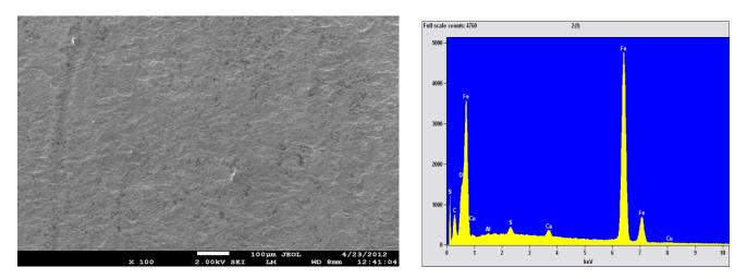
**Figure 4:** SEM micrograph of mild steel in 50% v/v *Arachis hypogeae*-2M H<sub>2</sub>SO<sub>4</sub> solution with the EDS spectrum
