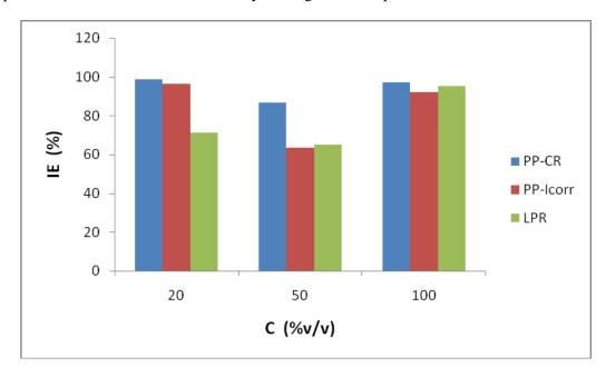
**Figure 5:** Comparative chart of inhibitor efficiency (IE) for 2M  $H_2SO_4$  solution/*Arachis hypogeae* concentration obtained from potentiodynamic polarization-corrosion rate (PP-CR), potentiodynamic polarization-corrosion current (PP-Icorr) and linear polarization resistance (LPR)
