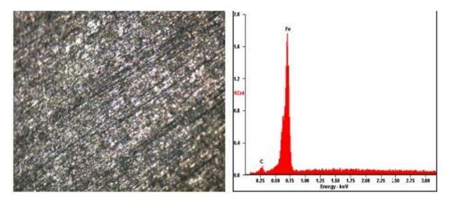
Figure 3: SEM micrograph of the as-received mild steel sample with the EDS spectrum
