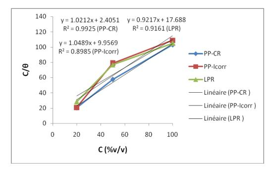
**Figure 6:** Langmuir isotherm for the adsorption of *Arachis hypogeae* compounds on the mild steel surface in  $2M H_2SO_4$  solution obtained from potentiodynamic polarization method at 298K
